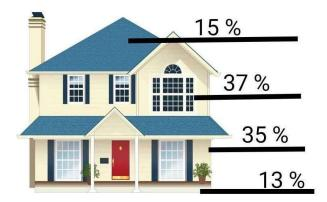
The building loses heat through all its parts, only the magnitude of the loss varies. About 35% of the heat is lost through the walls, 37% through the windows, 15% through the roof and 13% through the basement slab.
